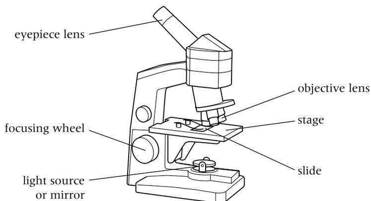
A microscope makes things appear bigger. It **magnifies** things. There are two **lenses** in a microscope. To work out the total **magnification** you multiply the magnification of the **objective lens** by the magnification of the **eyepiece lens**.
